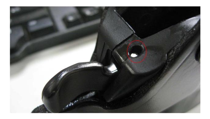
The dowel pin should be seated inside the molded housing with no signs of movement. The locking system should move freely and the handgun should holster in a locked position and draw without sticking upon release of the lever. If the handgun does not insert into the holster, or becomes locked or sticks in the holster during draw, immediately contact the Safariland Customer Care Department at (800) 347-1200 or (909) 923-7300.
